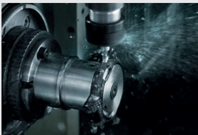
7. Redundant overlaying material is milled off and holes for pushers, the crown and the strap are milled into the case.
