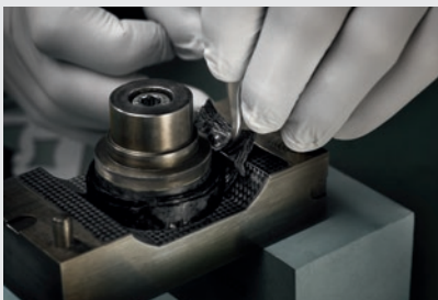
4. In the second phase all five pre-prepared parts are combined as one casting mould composition. No single layer is accidental or randomly oriented.
