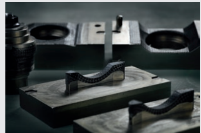
3. Each of the five parts is prepared by hand, and moulded and hardened separately. The five outer surfaces have their final finish.
