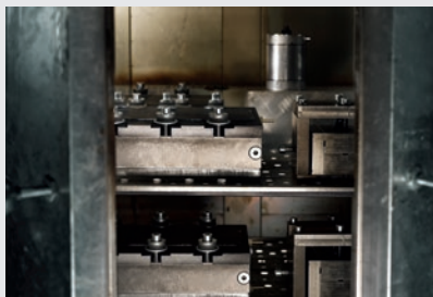
5. The casting mould composition is heated the second time up to 130 C and under 5 bar of pressure in special ovens.
