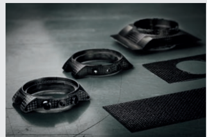
9. The evolution process shows the main stages of the production - from the woven carbon fibre reinforced polymer to the final case.
