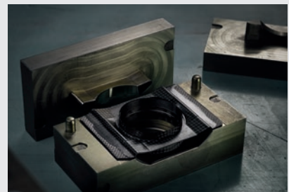
6. The case middle blank fuses all five single parts into one piece with up to 35 sheets of pre-cut woven carbon fibre reinforced polymer.
