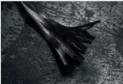
1. Flexible and thin carbon fibre reinforced polymer is the basis for the case.
